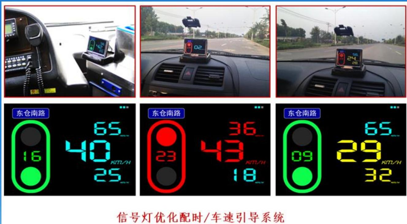
Optimized signal timing/Speed booting system
