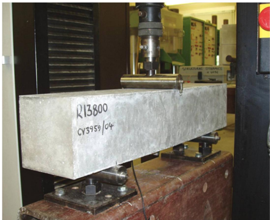
Test on beam of fibre-reinforced concrete with a notch
