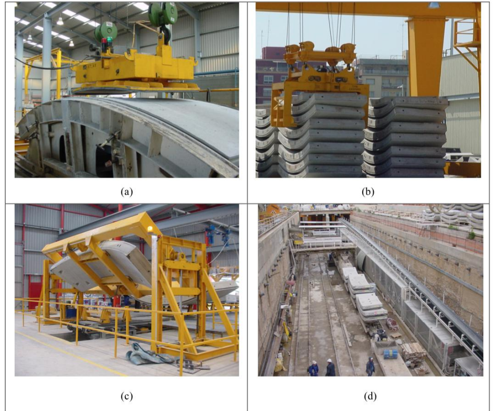
Figure 1. Transient load situations during production: (a) demoulding; (b) stacking; (c) handling and (d) transport
