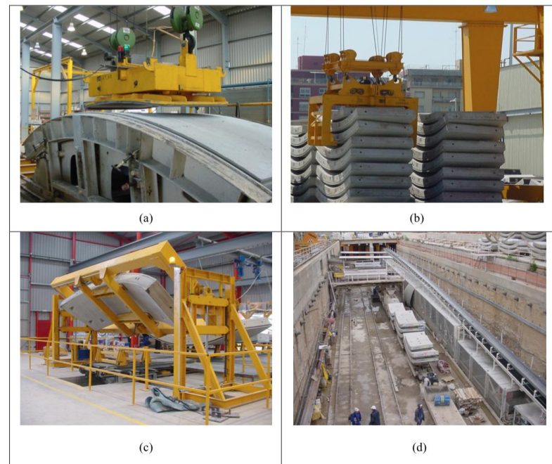
Figure 1. Transient load situations during production: (a) demoulding; (b) stacking; (c) handling and (d) transport
